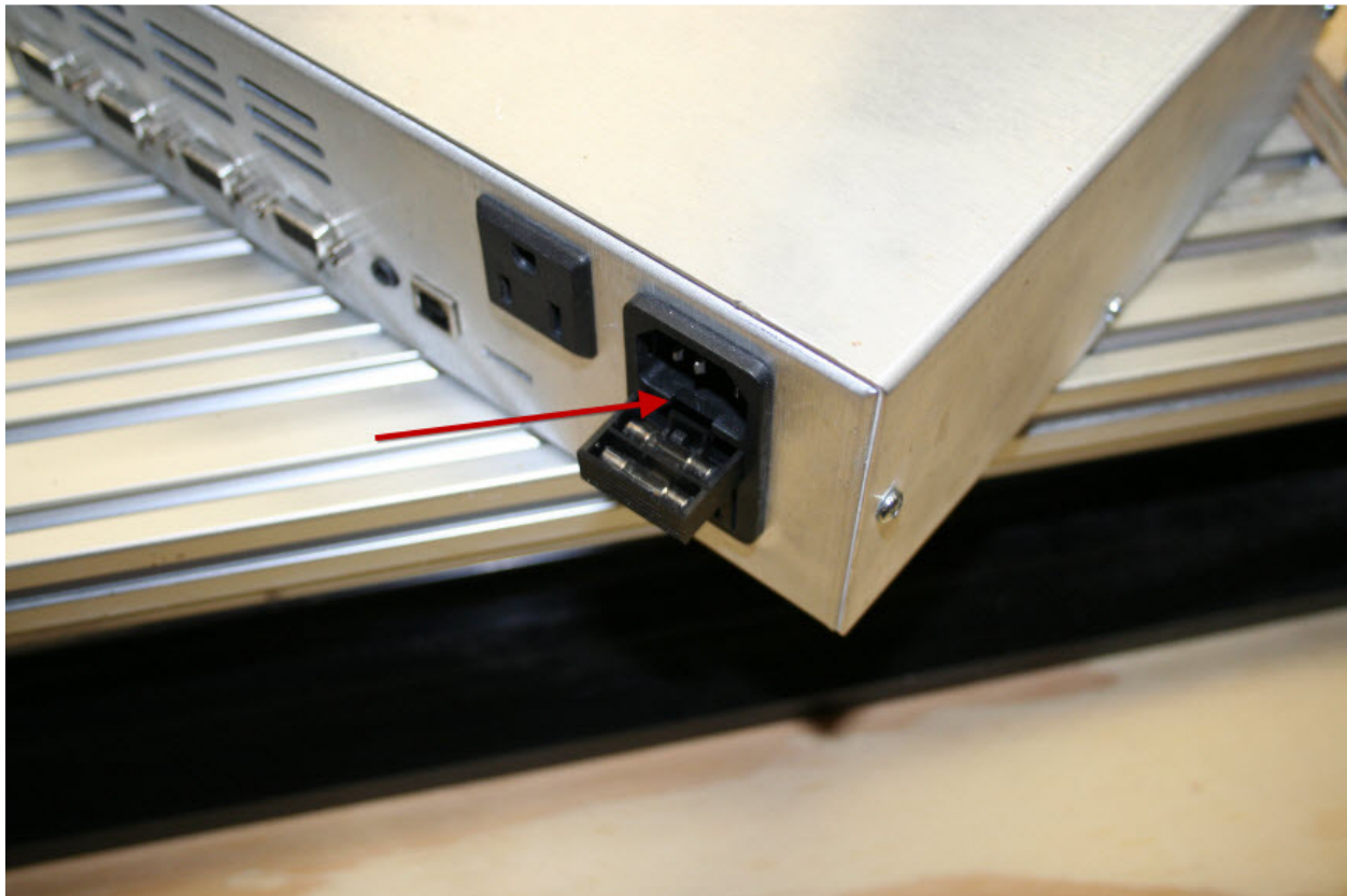
Figure 158 - Shark Control Box Power Cord Fuse
