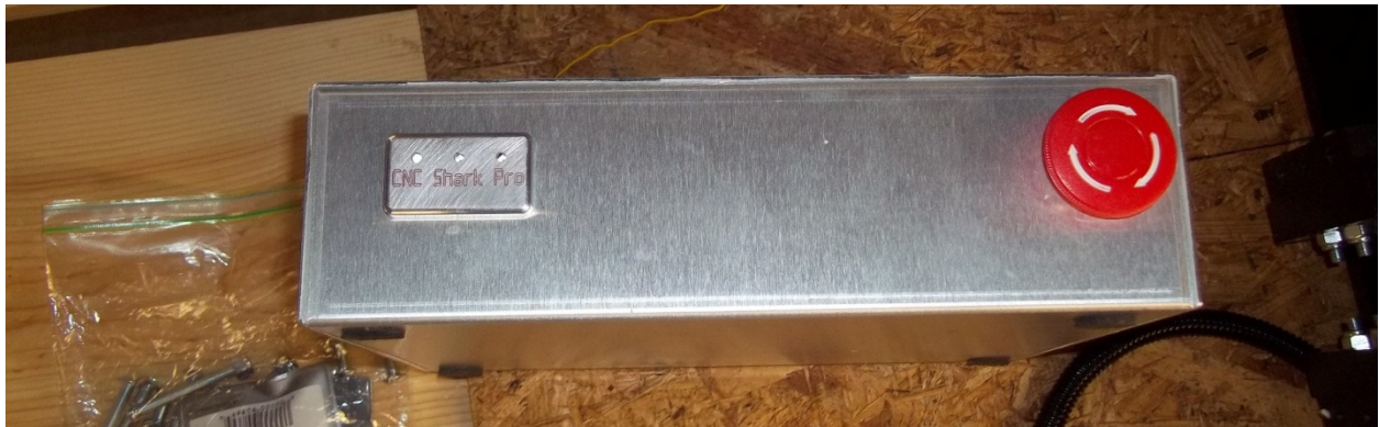
Figure 8 - CNC Shark Pro Plus and CNC Shark Pro Plus HD Enhanced Control Box Front Side
